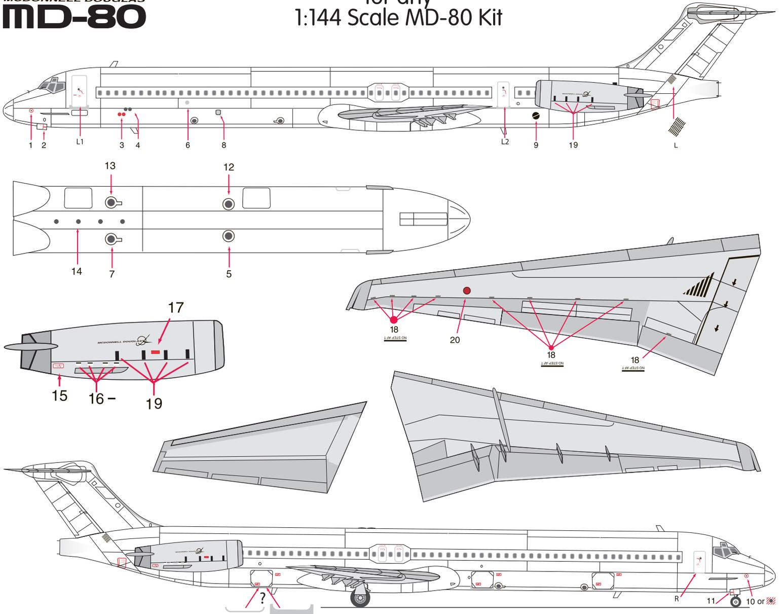
This McDonnell Douglas MD-80 Detail Sheet allows the modeler to apply stenciling and wing detailing to any version of the DC-9 Super 80 series of aircraft. Please keep in mind that stenciling data varies greatly from airline to airline and some small details may have been inadvertently left off while extra ones on the sheet may go unused for the particular aircraft you are modeling. Common grey and white door outlines have been provided, with 2 sets of white for better coverage.
